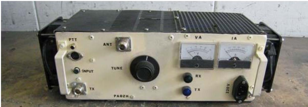
Its only 36 x 19 x 15 cm and the weight is not more than 5 kg. But there was a price to pay....the ring core transformer is a 800 volt type, 600 Kva at a duty cycle of 50%.
